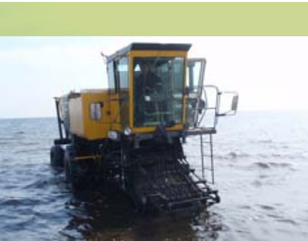
Test driving a marine harvester for algae outside Trelleborg.
